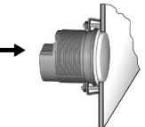
Place the flush mount seal on the instrument glass. Put the instrument into the drill hole from the back. Adjust the instrument so that the gauge is level and fasten it to the stud bolts (not included) on the rear side of the panel, using the flush mount fixing brackets.
