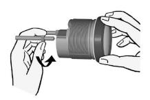
Place the bracket on the stud bolt and tighten the knurled nut. Do not over-tighten.
