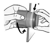
\* Make sure the seal lays flat between the panel and the front ring.
